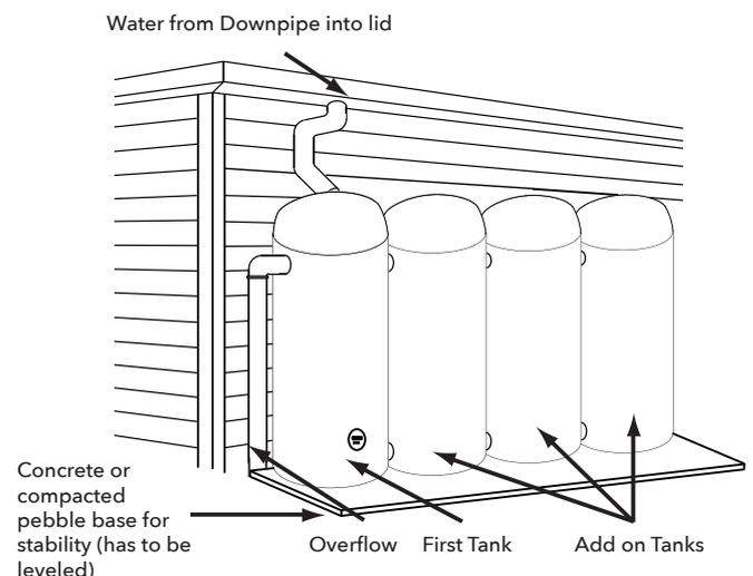
Cut hole for Downpipe into lid. A 98mm hole is required for wallace seal
