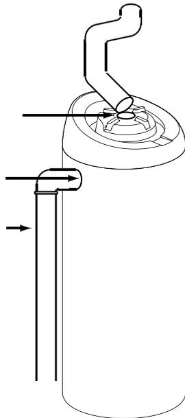
The tank comes already fitted with a 32mm fitting for the bottom outlet
