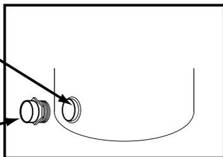
Attach a rubber adaptor to the fitting
